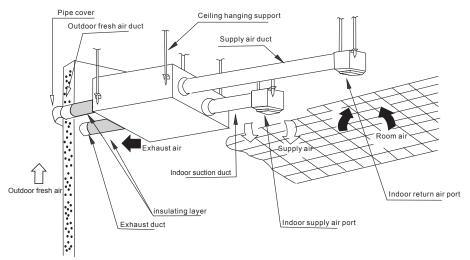
Two outdoor air ducts should keep warm to prevent condensation
