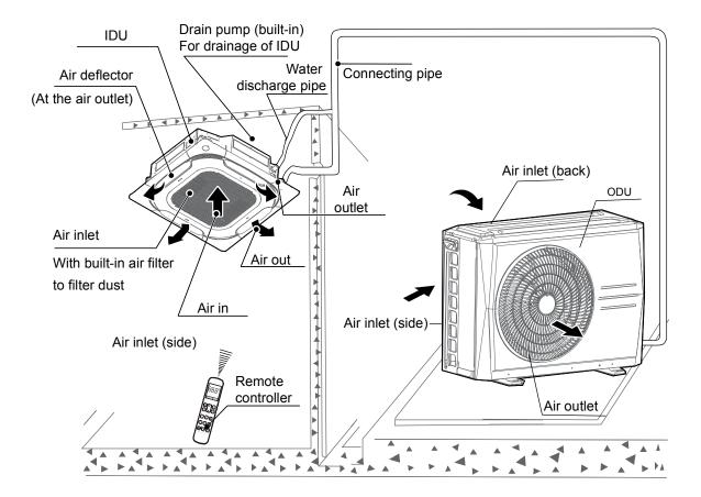
The air conditioner consists of the IDU, ODU, connecting pipe and wired/remote controller.
