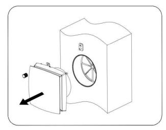
Loose the nut and pull the ventilator to remove.
