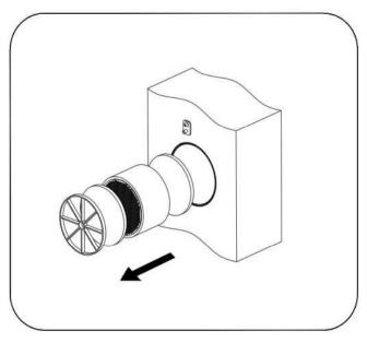
Remove the air flow rectifier Remove the filter in front of the regenerator.
