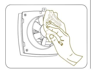
Clean the impeller blades. To remove dust use a soft brush, doth or a vacuum cleaner. Do not use water abrasive detergents, solvents, sharp objects. The impeller blades must be cleaned once in year.
