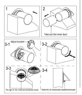
3. Through the wall hole from indoor, and pull back the duct by the adjust bracket to make the inner side rubber ring cling to the outside wall. Then put the inner duct in the hole and assembly inner duct and outer duct together. Fill the gap between the wall and duct with foam glue (Using waterproof sealing glue for the gap close to indoor to against rainwater). The inner duct should parallel with indoor wall surface.
