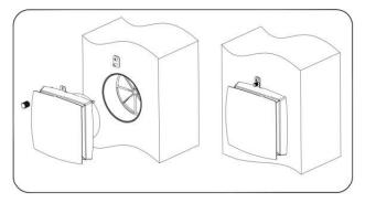
7. If you install the ventilator in the absence of rain, you can attach the rubber ring of the accessories bag to the out outer duct with the silicone glue. Don't fill the gap between the wall and duct with foam glue.
