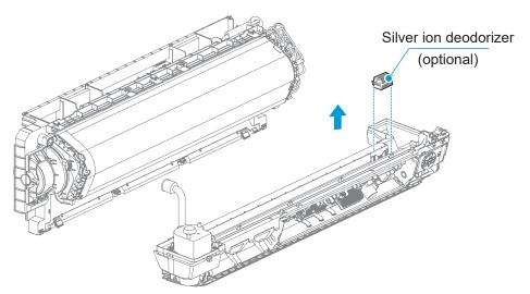
Loosen the screw (one), pull the evaporator horizontally a little and hang the evaporator.
