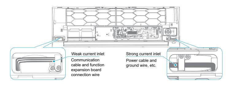
When there is a number of weak current wires, making it impossible for the cable clamp to fix all the wires, please use two ST3.6\*6.5 self-tapping screws to fix the power cable clamp from the accessory package on the installation board, and fix those weak current wires that cannot be fixed on the drain pan here.
