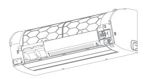
Loosen the screws inside the electric control box, remove the main control board and start repairing the unit.
