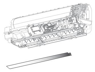
First loosen the screws (three) to remove the display panel, remove the cable terminal on the oscillation motor, then disconnect the left and right louver rod and the left and right swing motor rod, and take the swing motor and repair it.
