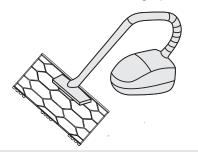
Clean the filter with clean water (except for the activated carbon module), with the air inlet side of the filter facing downwards.
