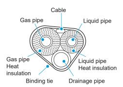
Note: If the drainage pipe is wrapped above the piping, it may cause poor drainage or backflow of water.
