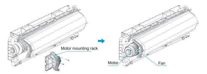
Take the motor and wind wheel out horizontally; loosen the screws fixing the motor and wind wheel, and repair the motor and wind wheel.
