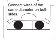
Do not press the power cables of the same wire diameter on the same side of the terminal. Do not use two power cables of different wire diameters for the same terminal blocks; otherwise, they can easily loosen due to uneven pressure and cause accidents, as shown in the figure below.
