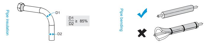
Note: D1 is the minimum diameter, and D2 is the nominal diameter.
