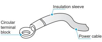
If it fails to crimp the insulated circular terminal block due to on-site limitations, connect the power cables of the same diameter to both sides of the power supply terminal block of the IDU, as shown in the figure below.
