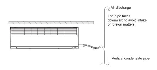
· Method to discharge water with the drain pump:
